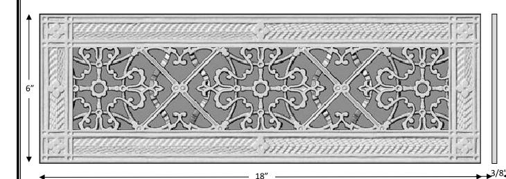
04" x 16" RR-209 04x16 to cover duct size finishes available 11 part number UPC Code | 731236368151 6" .9lb / 4lbs outside height weight / shipping weight 18" 3/8" **Arts & Crafts** outside width thickness style **Urethane Resin** 3-3/8" predrilled screw holes / screws 4/4 inside height material function | HVAC Grille inside width 15-3/8" free air flow 38.4 sq inch placement | Wall / Ceiling frame width 1-5/16" \$100 price
