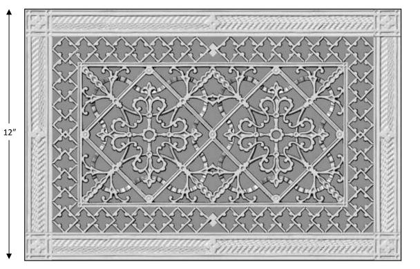
part number RR-209 10x16 10" x 16" to cover duct size finishes available 11 UPC Code **738759724334** 12" weight / shipping weight | 1.8lb / 6lbs outside height style | Arts & Crafts outside width 18" thickness 3/8" material Urethane Resin 9-3/8" predrilled screw holes / screws 4/4 inside height function HVAC Grille inside width 15-3/8" 106.7sq inch free air flow placement | Wall / Ceiling frame width 1-5/16" \$138 price
