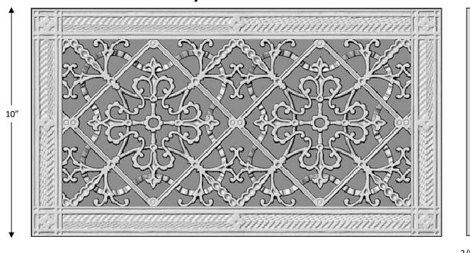
part number RR-209 08x16 to cover duct size 08" x 16" finishes available 11 UPC Code 731236368144 outside height 10" weight / shipping weight 1.6lb / 6lbs style **Arts & Crafts** outside width 18" thickness 3/8" **Urethane Resin** inside height 7-3/8" predrilled screw holes / screws 4/4 material function HVAC Grille inside width 15-3/8" 83.9sq inch free air flow placement Wall / Ceiling frame width 1-5/16" price \$122
