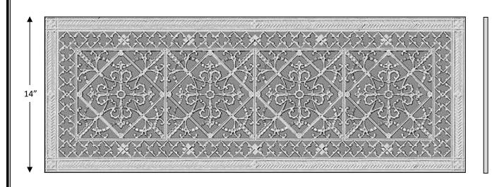
part number RR-209 12x36 12" x 36" finishes available | 11 to cover duct size 14" 3.6lb / 16lbs UPC Code | 731236369912 outside height weight / shipping weight style | Arts & Crafts outside width 38" thickness 3/8" material Urethane Resin 11-3/8" free air flow 297.8sq inch inside height function | HVAC Grille 35-3/8" inside width predrilled screw holes / screws 6/6 placement | Wall / Ceiling frame width 1-5/16" \$341
